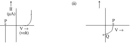
a) Name the type of a diode whose characteristics are shown in the figure (i) and figure (ii).
